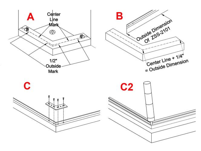
Screws. Now place the assembled Curb pieces in the position laid out on the shower curb corresponding to the marks that you made. Make sure to fill the corners where the screws were inserted and the ends with silicone so as to seal any gaps that might leak but do this after the wall jams are installed (C).
