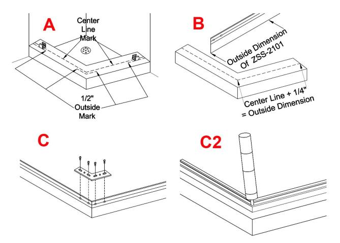
Screws. Now place the assembled Curb pieces in the position laid out on the shower curb corresponding to the marks that you made. Make sure to fill the corners where the screws were inserted and the ends with silicone so as to seal any gaps that might leak but do this after the wall jams are installed **(C)**.
