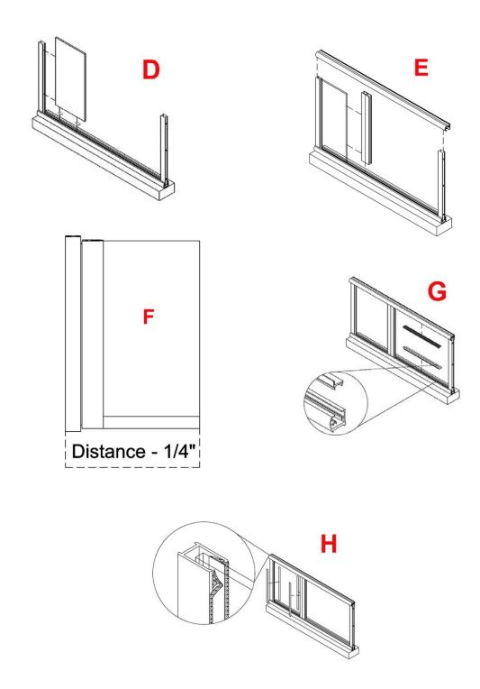
out. Notice the locking groove. Do not stretch either vinyl as they will shrink over time creating gaps where water can get into (I). At step 11 caulk all the joints where vertical vinyl meets horizontal vinyl.
