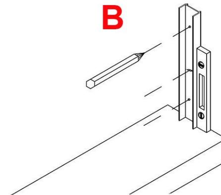
**2)** Now drill the 3 holes with a 3/16" masonry bit (9/64" regular bit for fiberglass, & without anchors). Then insert the 3)-ZV935 screw anchors (#2) in the holes. Fasten the ZTE1203 wall jambs in place using the #8X1-1/4 Phillips Pan Head screws provided (#3) **(C)**. **Important Note:** The ZV926 Bottom Bumper (#4A) needs to be installed with the bottom screw on the jamb, on
