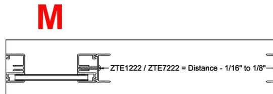
the underneath of the ZTE-1222 Curb (N). Slide the curb down between the wall jambs and onto the tub/shower. Make sure the curb is solid and doesn't rock back and forth. If it is not solid secure it with two of the #6X3/8" Pan Head Screws (#13) provided by drilling with a 1/8" drill bit through the outside leg of the wall jamb at the bottom, into the face of the curb and inserting the screws (O).
