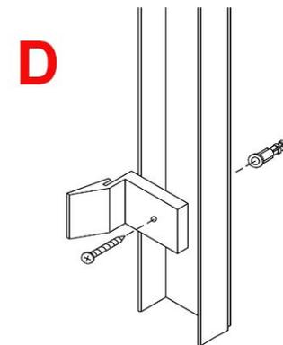
the showerhead side of the unit, with the angled side of the bumper going to the inside of the shower. Refer to the exploded view. Attach one of the ZV924 Bumpers (#4) using the #6/32X1/2 Machine screws (#5) keeping in mind that the inside panel will be on the showerhead side of the shower **(D)**.
