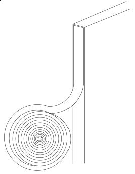
Then remove protective layer from other side and attach seal to the tape surface. Press on by hand. Cut flush to the bottom of the door using pliers-type cutter, scissors, or razor knife. The VHB tape will gain strength and achieve full bond within 72 hours.
