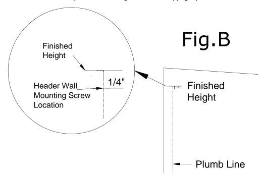
This will be the location of the wall mounting screw(Fig.C).
