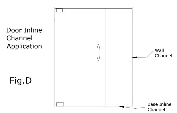
Base inline channel: bottom dimension of inline panel + 5/16"
