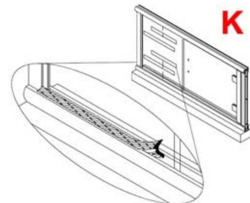
**7)** Now you need to cut the Snap In Filler ZSS2102 (#4). There are a number of ways to calculate the size of the ZSS2102. This simple method will work for standard width as well as custom. Measure the distance in-between the edge of the glass panel and the ZD8004 "Door Hinge Jamb". This will be the size of your ZSS2102. Cut to that Dimension (**L**).
