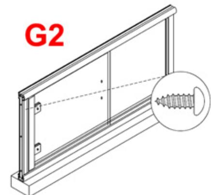
**5)** Securing the header and curb. Drill a  $1/8"$  hole on the inside through the ZSS2101 header into the ZD1006. (**I**).
