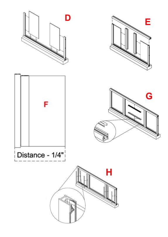
between the glass and the curb, and the glass and the header (top and bottom) inside and out. Notice the locking groove. Do not stretch either vinyl as they will shrink over time creating gaps where water can get into. At step 11, caulk all the joints where vertical vinyl meets horizontal vinyl. (1)
