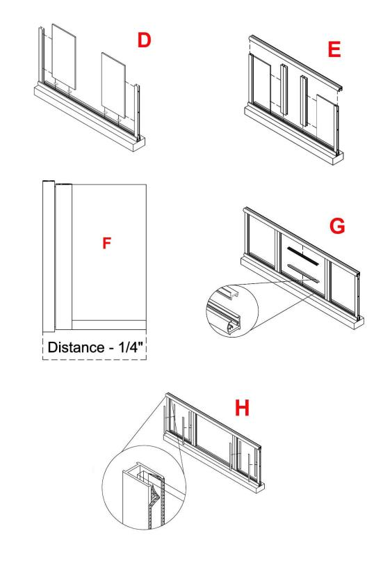
between the glass and the curb, and the glass and the header (top and bottom) inside and out. Notice the locking groove. Do not stretch either vinyl as they will shrink over time creating gaps where water can get into. At step 11, caulk all the joints where vertical vinyl meets horizontal vinyl. (1)
