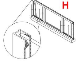
between the glass and the curb, and the glass and the header (top and bottom) inside and out. Notice the locking groove. Do not stretch either vinyl as they will shrink over time creating gaps where water can get into. At step 11, caulk all the joints where vertical vinyl meets horizontal vinyl. (1)
