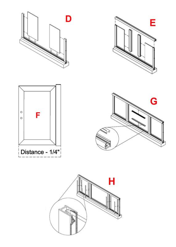
and the header (top and bottom) inside and out. Notice the locking groove. Do not stretch either vinyl as they will shrink over time creating gaps where water can get into (I). At step 11 caulk all the joints where vertical vinyl meets horizontal vinyl.
