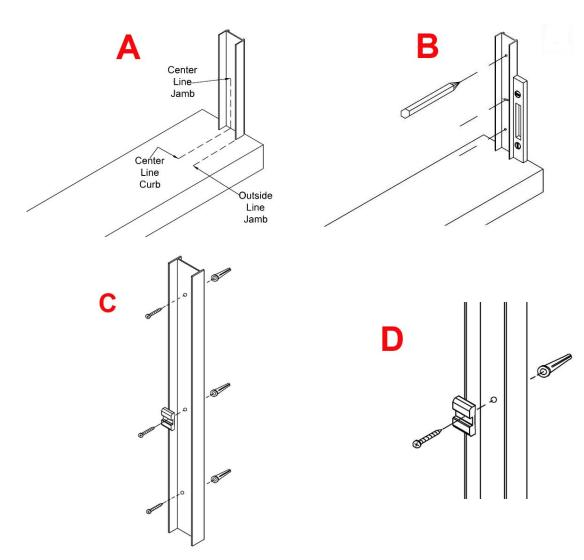
screws of the wall jambs **(D)**. Refer to the exploded view drawing.
