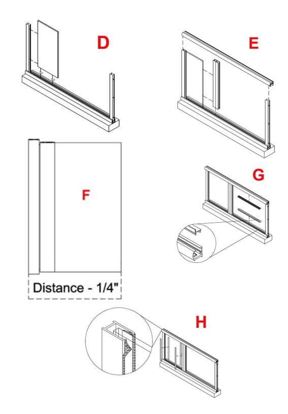
bottom) inside and out. Notice the locking groove. Do not stretch either vinyl as they will shrink over time creating gaps where water can get into. At step 11, caulk all the joints where vertical vinyl meets horizontal vinyl. (I)
