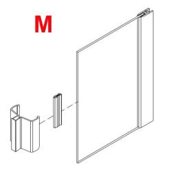
**10)** Cut the Bottom Poly Rail (ZVP-316WS for 3/16" glass, ZVP-14WS for 1/4" glass) then push over the bottom edge of the glass. Run a cap bead of silicone on the inside where the glass and poly meet to prevent water seeping down into the sweep between the glass and poly (N).
