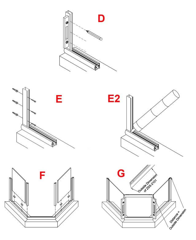
door header. Mark the Header at that dimension and cut. Repeat the procedure for the other ZSS-2101 Header (G).
