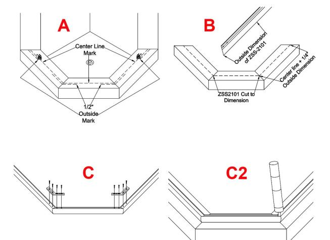
screws and then place the assembled Curb in the position laid out on the shower curb, corresponding to the marks that you made. Make sure to fill the corners where the screws were inserted and the ends with silicone so as to seal any gaps that might leak but do this after the wall jams are installed (C).
