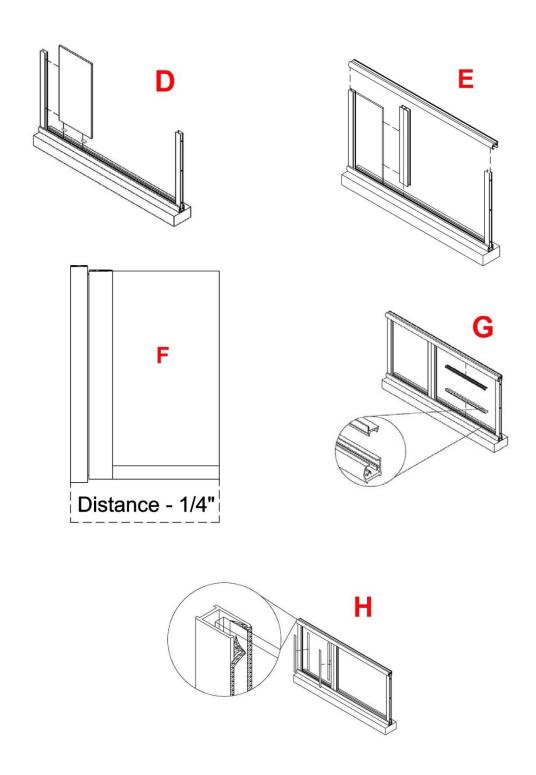
bottom) inside and out. Notice the locking groove. Do not stretch either vinyl as they will shrink over time creating gaps where water can get into. At step 11 caulk all the joints where vertical vinyl meets horizontal vinyl. (1)
