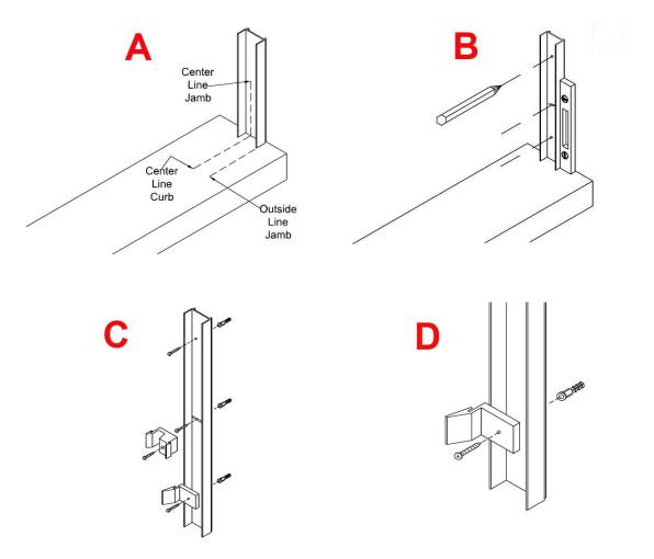
the showerhead side of the unit, with the angled side of the bumper going to the inside of the shower. Refer to the exploded view. Attach one of the ZV924 Bumpers (#4) using the #6/32X1/2 Machine screws (#5) keeping in mind that the inside panel will be on the showerhead side of the shower(**D**).
