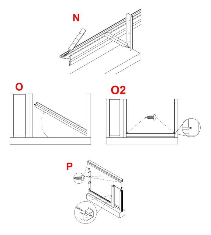
would be valuable at this point to hold the inside panel on an angle toward the inside so the outside panel can be lowered and positioned to be installed into the outside roller track. The inside panel will be positioned at the showerhead side of the shower while the outside panel will be positioned opposite the showerhead. This is to ensure that no water escapes through the overlap (Q).
