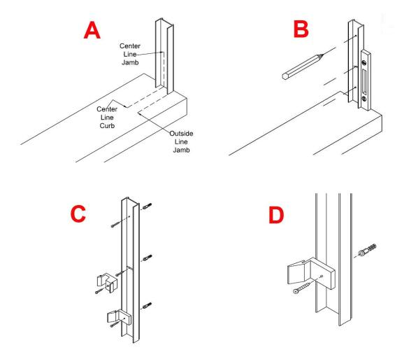
the showerhead side of the unit, with the angled side of the bumper going to the inside of the shower. Refer to the exploded view. Attach one of the ZV924 Bumpers (#4) using the #6/32X1/2 Machine screws (#5) keeping in mind that the inside panel will be on the showerhead side of the shower (D).
