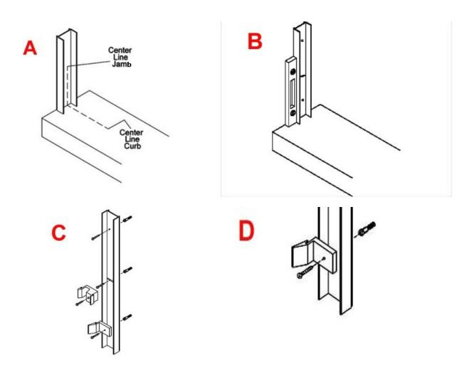
the ZV924 Bumpers (#4) using the 2-#6/32X1/2 Machine screws (#5) keeping in mind that the inside panel will be on the showerhead side of the shower.
