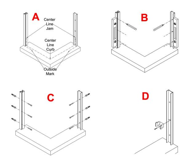
using the #8X1-1/4 Phillips Pan Head screws provided (#13) **(C)**. **Important Note:** The ZV926 Bottom Bumper (#4A) needs to be installed with the bottom screw on the ZTE-1203 Jamb, on the showerhead side of the unit, with the angled side of the bumper going to the inside of the shower. Refer to the exploded view. Attach one ZV924 Bumper (#4) on the ZTE-1203 using the #6/32X1/2 Machine screw (#5) keeping in mind that the inside panel will be on the showerhead side of the shower **(D)**.
