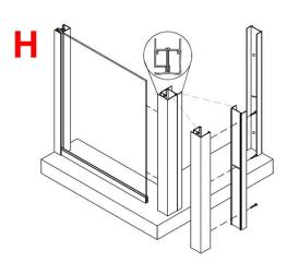
1" screw depending on the model). Place the 90 Post which consists of a ZTE-1203 Wall Jamb (#1) and a ZTE-1214 90 Jamb Post (#20) attached together, over the edge of the glass (H). Adjust the 90° post to be plumb from both directions. Insert the ZV909 Wedge Vinyl (#19) into the jambs on both sides of the glass. A block of wood will help push the vinyl in. Slightly wet the vinyl with water to ease install. The flat side goes against the glass (I).
