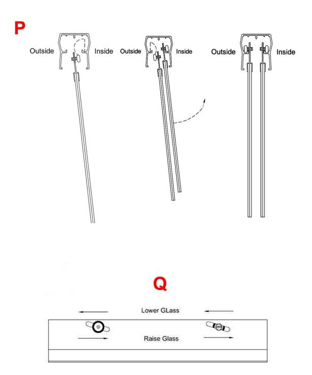
just to the side of the panels, slip the front lip in, then snap the guide down over the inside of the curb. Slide the guide over carefully. When the doors are in a closed position the center guide should be centered in the overlap of the glass. For added security you can attach the guide after it is snapped in place by drilling with a 1/8" drill bit through the snap in leg and into the curb (from the inside of the shower) then running a #6X3/8 screw into the hole (R).
