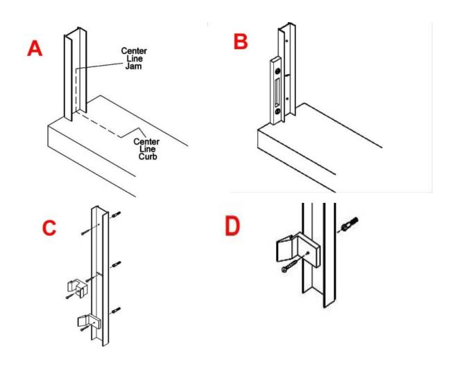
the ZV924 Bumpers (#4) using the 2-#6/32X1/2 Machine screws (#5) keeping in mind that the inside panel will be on the showerhead side of the shower.
