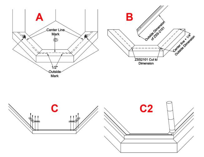
screws and then place the assembled Curb in the position laid out on the shower curb, corresponding to the marks that you made. Make sure to fill the corners where the screws were inserted and the ends with silicone so as to seal any gaps that might leak but do this after the wall jams are installed (C).
