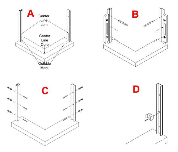
using the #8X1-1/4 Phillips Pan Head screws provided (#13) **(C)**. **Important Note:** The ZV926 Bottom Bumper (#4A) needs to be installed with the bottom screw on the ZTE-1203 Jamb, on the showerhead side of the unit, with the angled side of the bumper going to the inside of the shower. Refer to the exploded view. Attach one ZV924 Bumper (#4) on the ZTE-1203 using the #6/32X1/2 Machine screw (#5) keeping in mind that the inside panel will be on the showerhead side of the shower **(D)**.
