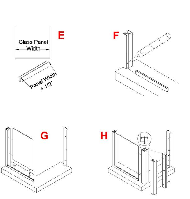
1" screw depending on the model). Place the 90 Post which consists of a ZTE-1203 Wall Jamb (#1) and a ZTE-1214 90 Jamb Post (#20) attached together, over the edge of the glass (H). Adjust the 90° post to be plumb from both directions. Insert the ZV909 Wedge Vinyl (#19) into the jambs on both sides of the glass. A block of wood will help push the vinyl in. Slightly wet the vinyl with water to ease install. The flat side goes against the glass (I).
