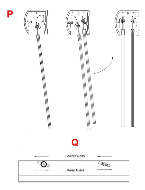
just to the side of the panels, slip the front lip in, then snap the guide down over the inside of the curb. Slide the guide over carefully. When the doors are in a closed position the center guide should be centered in the overlap of the glass. For added security you can attach the guide after it is snapped in place by drilling with a 1/8" drill bit through the snap in leg and into the curb (from the inside of the shower) then running a #6X3/8 screw into the hole **(R)**.
