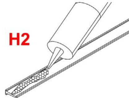
**7)** Cut the Bottom Poly Rail (ZVP-14WS for 1/4" glass (#22)) then push over the bottom edge of the glass. Run a cap bead of silicone on the inside where the glass and poly meet to prevent water seeping down into the sweep between the glass and poly. **(Note:** to ensure that the door will close completely, notch out the section of plastic that makes contact with the ZD8004 "Magnetic Latch Jamb") **(I)**.
