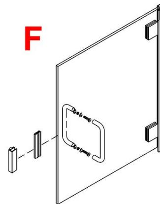
**5)** Place a small amount of silicone on the legs of the 2-ZV940 Door Clips (#20) and place down into the top of the 1006's to cap the opening. You may have to trim them to fit with side cutters **(G)**.
