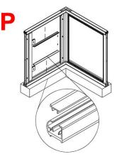
**9)** Cut the Bottom Poly Rail (ZVP-316WS for 3/16" glass, ZVP-14WS for 1/4" glass) then push over the bottom edge of the glass. Run a cap bead of silicone on the inside where the glass and poly meet to prevent water seeping down into the sweep between the glass and poly **(Q)**.
