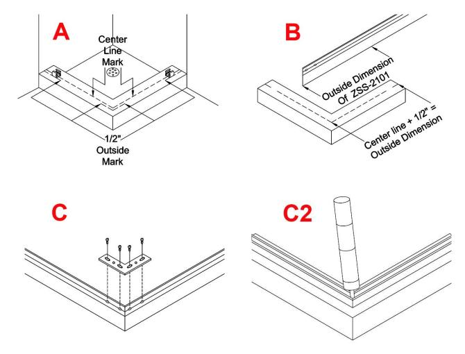
corresponding to the marks that you made. Make sure to fill the corner where the screws were inserted and ends with silicone so as to seal any gaps that might leak **(C)**.
