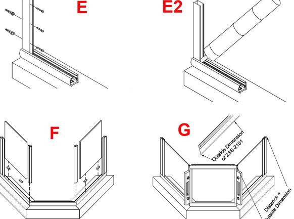
door header. Mark the Header at that dimension and cut. Repeat the procedure for the other ZSS-2101 Header (G).
