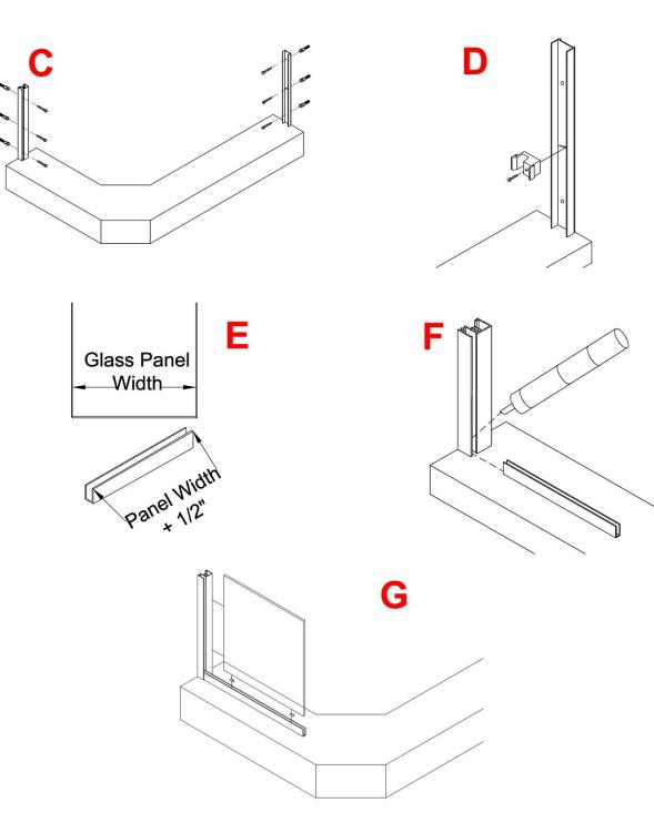
Slightly wet the vinyl with water to ease install. The flat side goes against the glass (H).
