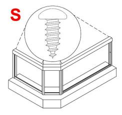
panels are installed the inside panel will be positioned at the showerhead side of the shower while the outside panel will be positioned opposite the showerhead. This is to ensure that no water escapes through the overlap (T).
