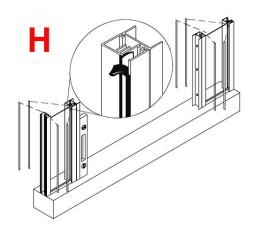
the vertical jambs on both sides. A block of wood will help push the vinyl in. Wet the vinyl slightly with water to ease install. The flat side goes against the glass. Make sure the posts are plumb (H). Repeat this process for the other panel on the opposite side.
