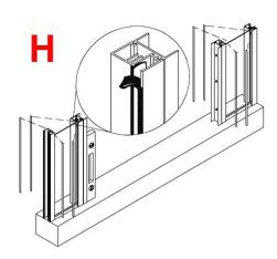
the vertical jambs on both sides. A block of wood will help push the vinyl in. Wet the vinyl slightly with water to ease install. The flat side goes against the glass. Make sure the posts are plumb (H). Repeat this process for the other panel on the opposite side.
