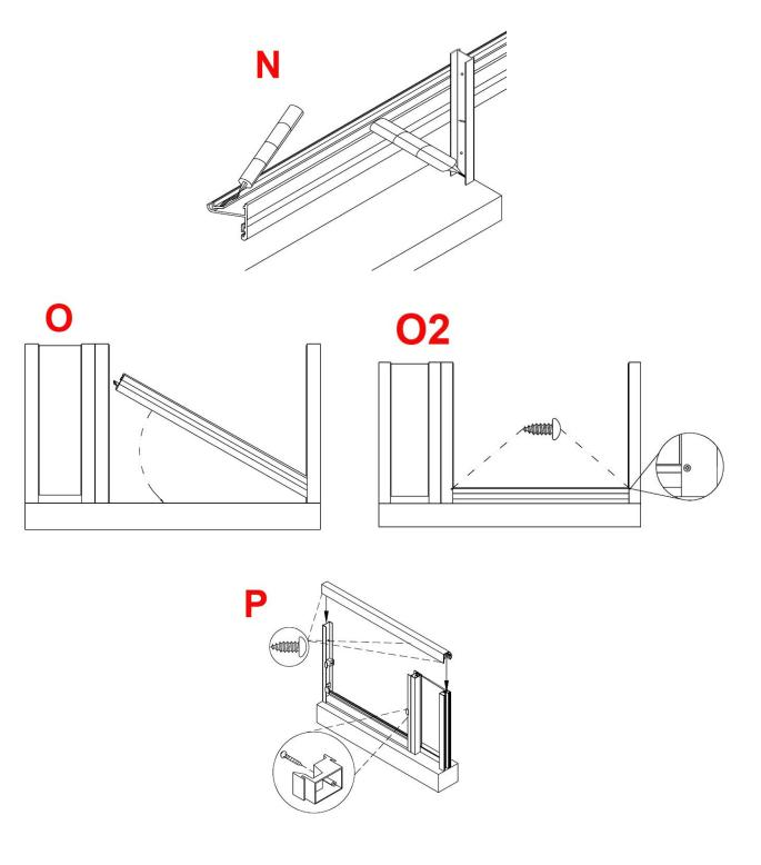
positioned to be installed into the outside roller track. The inside panel will be positioned at the showerhead side of the shower while the outside panel will be positioned opposite the showerhead. This is to ensure that no water escapes through the overlap (Q).
