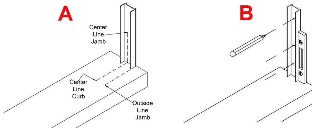
**2)** Now drill the 3 holes with a 3/16" masonry bit (9/64" regular bit for fiberglass, & without anchors). Then insert the 3)-ZV935 screw anchors (#2) in the holes. Fasten the ZTE1203 wall jambs in place using the #8X1-1/4 Phillips Pan Head screws provided (#3) **(C)**. **Important Note:** The ZV926 Bottom Bumper (#4A) needs to be installed with the bottom screw on the jamb, on
