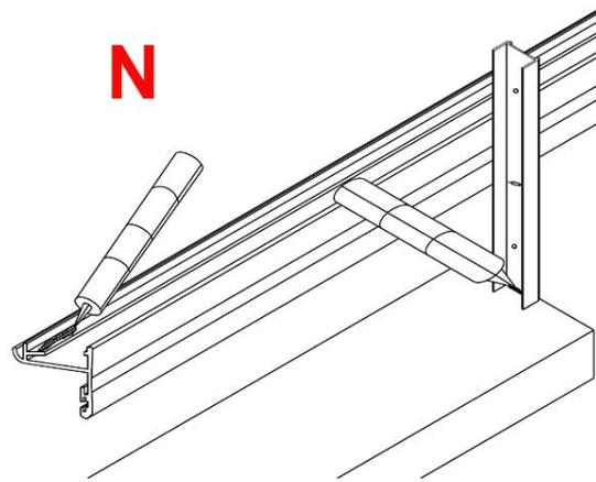
8) Plumb the 180° Jamb/Post (#9) and attach the header to the Jambs and Post from the inside of the shower using #6 x 3/8" Phil Pan Head Screws (#13). Attach the other ZV924 Bumper (#4) using the #6/32X1/2 Machine screw (#5) keeping in mind that the inside panel will be on the showerhead side of the shower (P).
