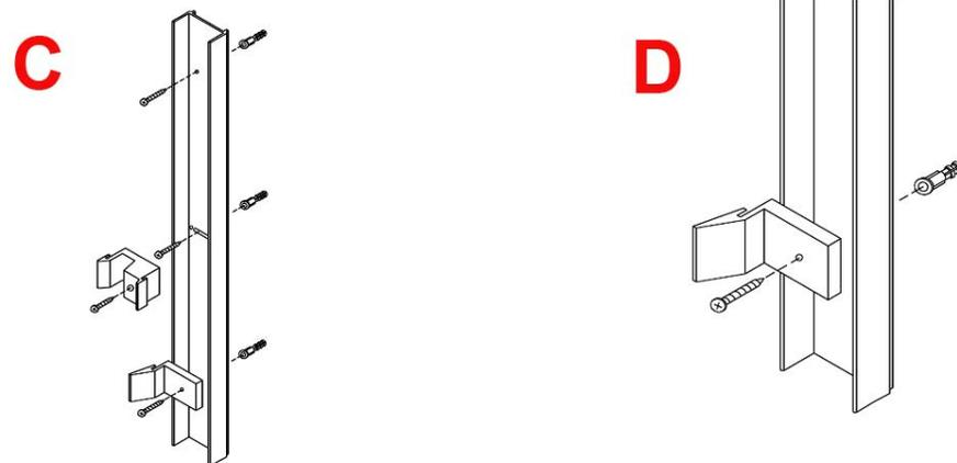
the showerhead side of the unit, with the angled side of the bumper going to the inside of the shower. Refer to the exploded view. Attach one of the ZV924 Bumpers (#4) using the #6/32X1/2 Machine screws (#5) keeping in mind that the inside panel will be on the showerhead side of the shower **(D)**.
