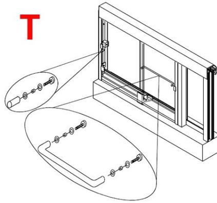
**13)** Attach the towel bar on the outside panel with two holes using the same method as the knob in step 7 **(T)**.
