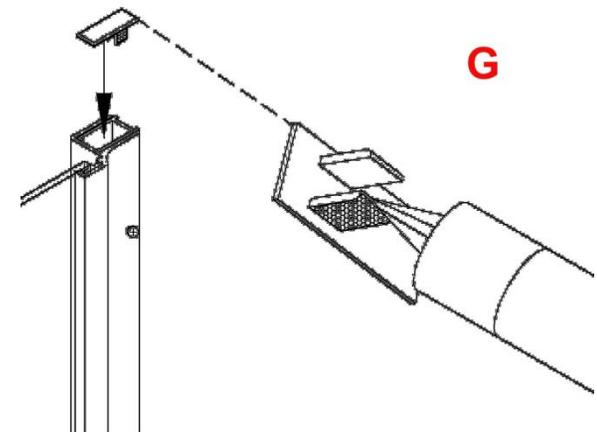
**5)** Place a small amount silicone on the legs of the 2-ZV940 Door Clips (#20) and place down into the top of the 1006's to cap the opening. You may have to trim them to fit with side cutters. **(G)**
