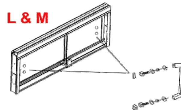
**8)** Attach the second ASDSQ8 (#9) handle **(M)** on the outside panel using the same method as in step 7. This handle should be on the outside of the unit opposite the showerhead.
