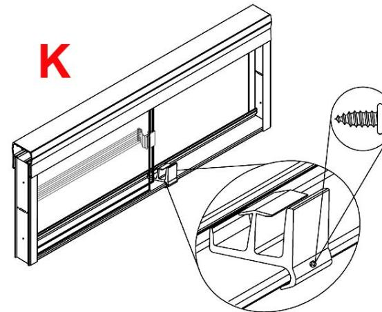
**7)** Attach the Handle ZTE1207-3 (#12) (**L**) by placing the Handle Gasket ZV916 (#14) over the edge of the glass aligning it with the middle wall jamb bumper (ZV924) on the shower head side panel. Then place the handle over the gasket and gently tap onto the glass with a rubber mallet.
