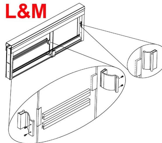
**8)** Attach the Towel Bar (**M**) using the ZTE1206-3 (#9) and the ZTE1206P-3 (#10) Brackets. Follow the same procedure as step 7 aligning the brackets with the middle wall jamb bumper. The 1206P will be used on the wall jamb side of the towel bar while the 1206 will go on the overlap side. After you attach the brackets slide the Towel Bars ZTE1205 (#11) into the brackets and secure with 4-#6X3/8 screws.
