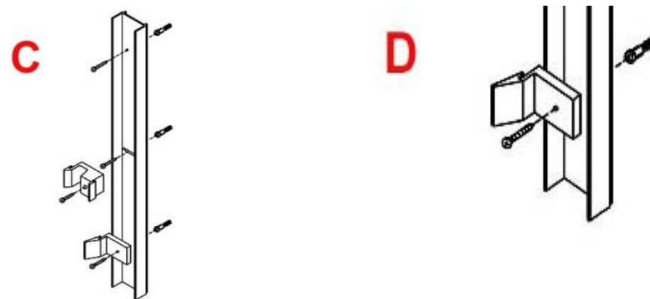
the ZV924 Bumpers (#4) using the 2-#6/32X1/2 Machine screws (#5) keeping in mind that the inside panel will be on the showerhead side of the shower.
