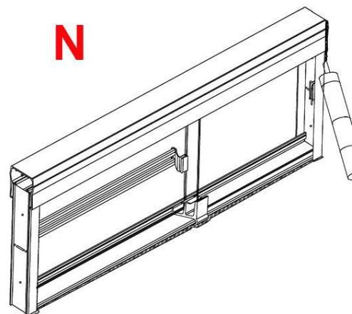
**9)** Run a bead of silicone on the gap between the metal and the shower surface inside and out. Fill all joints and gaps where metal meets metal and fill with a fine bead. (**N**)
