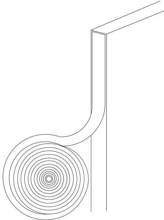
Then remove protective layer from other side and attach seal to the tape surface. Press on by hand. Cut flush to the bottom of the door using pliers-type cutter, scissors, or razor knife. The VHB tape will gain strength and achieve full bond within 72 hours.
